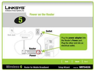
Figure 6-7: Power on the Router Screen
